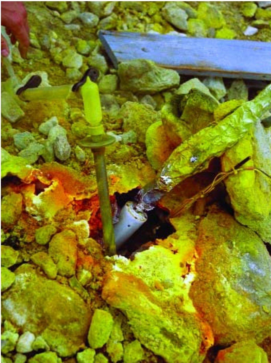
Figure 3. Photograph of the evanescent field fiber sensor inserted into a volcanic fumarole. The titanium tube for simultaneous collection of gas samples and a temperature sensor can also be seen.
