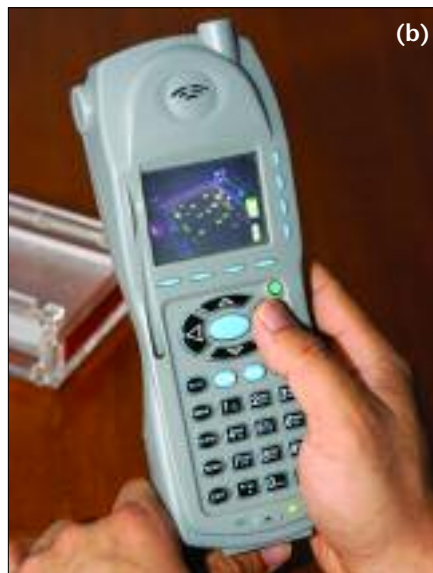
Figure 2. Illustration of Spectrosity's handheld electrophoresis device, the DigiPAC (a) and the actual prototype (b). Spectrosity designed the product for the higher education market.
