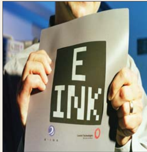
Figure 2. Two electronic paper technologies have been commercialized. (a) Gyricon consists of 75-100 \mu\text{m} bichromal spheres (left) that are individually encapsulated in a polymer matrix to form a flexible display (right) [Courtesy Gyricon]. (b) E-Ink consists of closely packed capsules filled with micrometer-sized charged particles (left) that can be sandwiched between two flexible substrates (right) [Courtesy E-Ink Corp].
