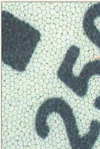
Figure 2. Two electronic paper technologies have been commercialized. (a) Gyricon consists of 75-100 \mu\text{m} bichromal spheres (left) that are individually encapsulated in a polymer matrix to form a flexible display (right) [Courtesy Gyricon]. (b) E-Ink consists of closely packed capsules filled with micrometer-sized charged particles (left) that can be sandwiched between two flexible substrates (right) [Courtesy E-Ink Corp].
