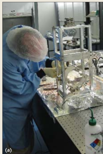
(Left to right) Florian English, Brian Orr (CLA Director) and Yabai He with a continuous-wave cavity ringdown spectrometer for multiwavelength molecular sensing.
