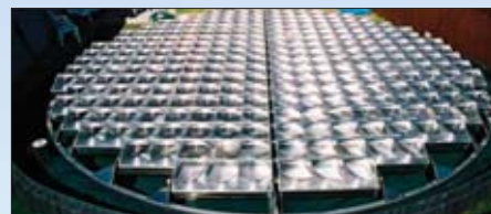
Prototype of concentrator system made by Pyron. The system stays aligned with the sunlight by pivoting along each row of lenses and rotating around the circular ring.
