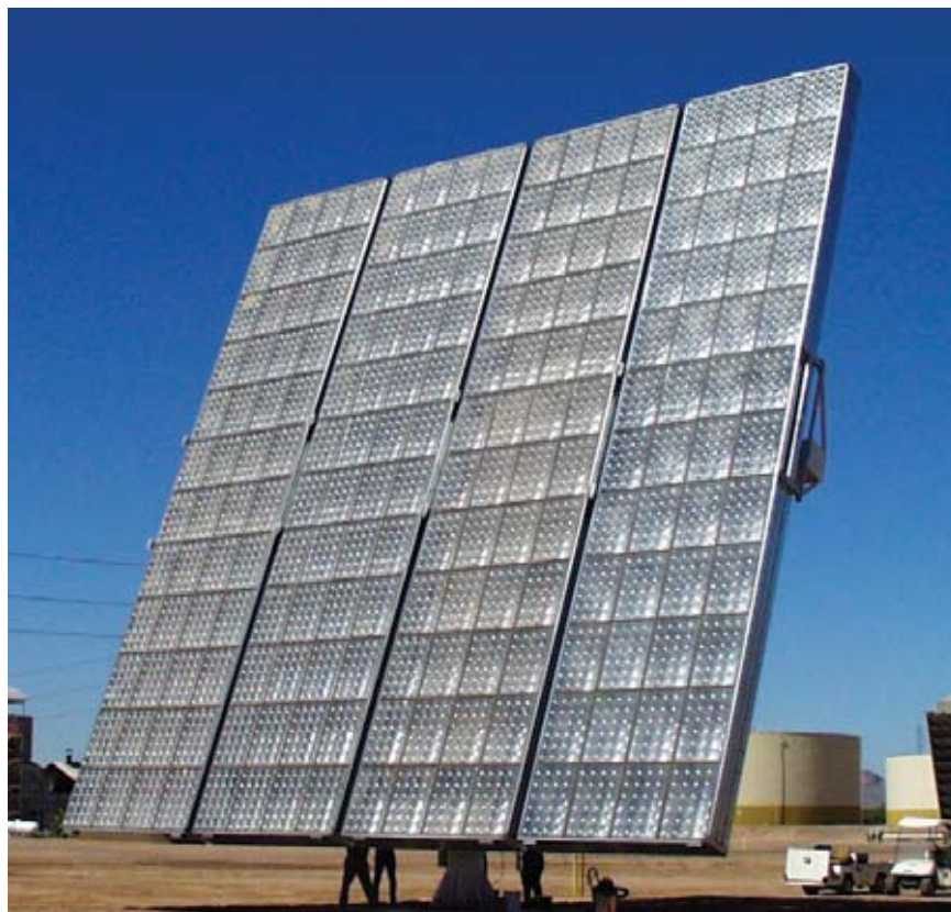
Figure 3. Amonix system installed at Arizona Public Service's site in Phoenix, Ariz. The Amonix systems use an array of Fresnel lenses to focus light on silicon cells that are distributed across the backplane.
